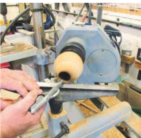
STEP 17. I have seen many ways of removing the shavings/dust from inside a piece, including methods such as spoons, vacuum cleaners and even straws. Compressed air works the best – just watch your eyes as it ejects from the opening
